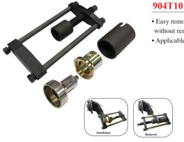
2/18/19.5/0.5 ∆ ∆ 9250g • Easy removal and replacement of the rear trailing arm bushes without removing the trailing arm completely from the vehicle. • Applicable : Mazda - PREMACY CREW/CR3W (05~10), AXELA (03-09), 3 - BK (03~08), BL (09~), 5- CR (05~10) Ford - C-MAX CAP (03-07), FOCUS I (98-05), KUGA CBV FOCUS II (04-08) FOCUS CB4 (08-11) Volvo - S40 II / V50 (04-12)
